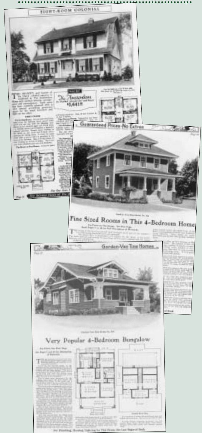
Catalog pages showing exteriors and floor plans. Sears “Amsterdam,” a Dutch Colonial; a Gordon-Van Tine four square; and a Gordon-Van Tine bungalow.
